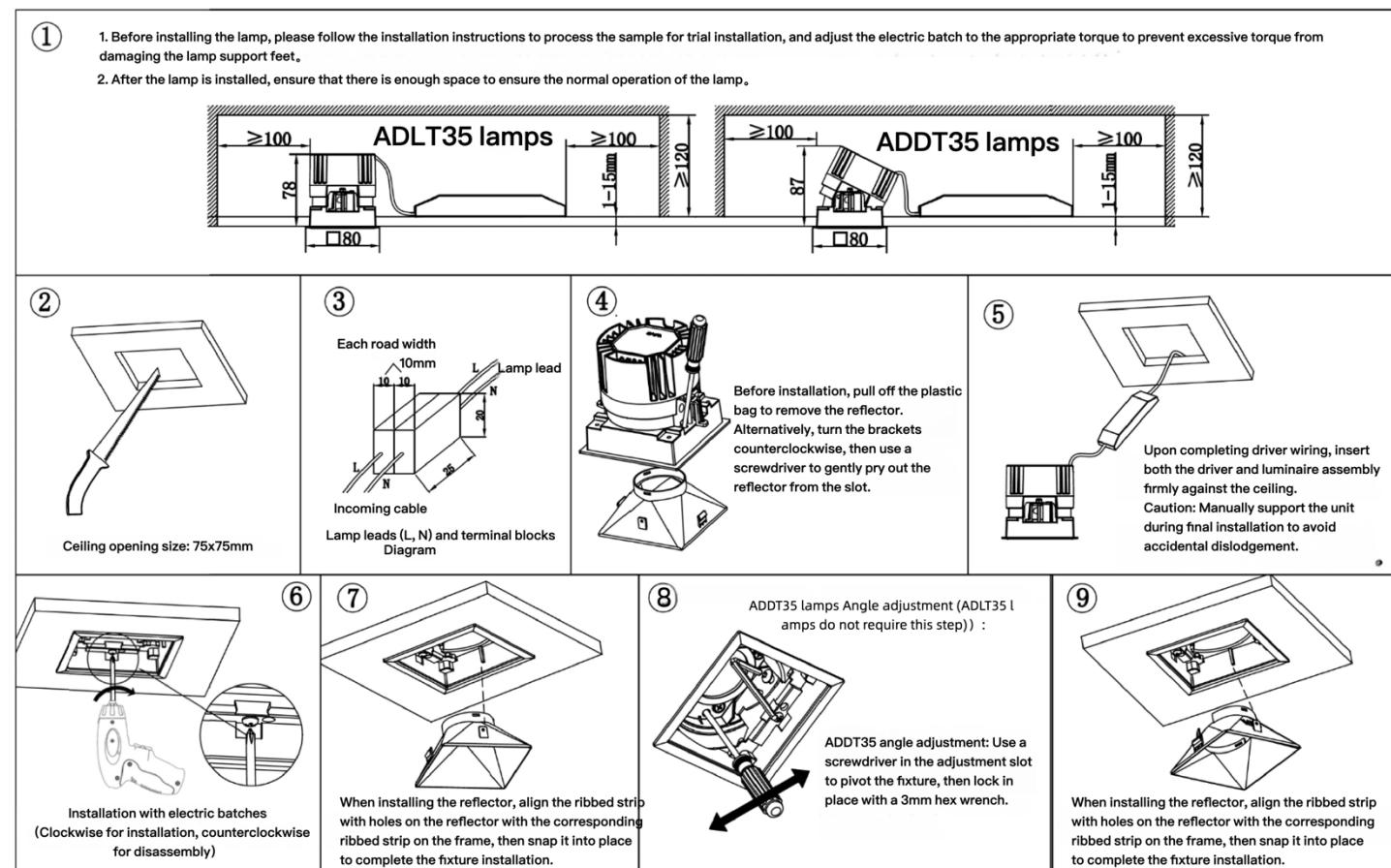
\* If the lighting fixture has built-in leads, and these connection leads need to be connected to an independent terminal block (refer to Figure 5 for connection diagram), each terminal block size should not be less than 10x20x25mm.
