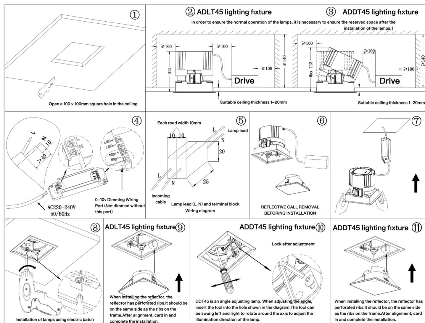
\* If the lighting fixture has built-in leads, and these connection leads need to be connected to an independent terminal block (refer to Figure 5 for connection diagram), each terminal block size should not be less than 10x20x25mm.
